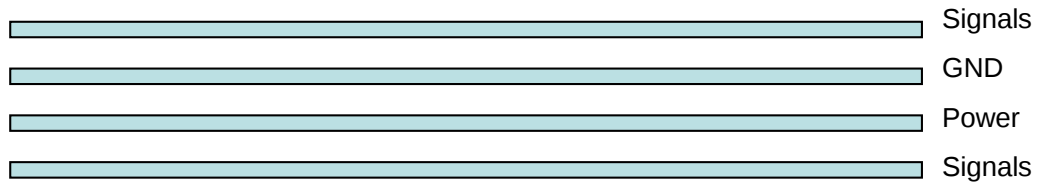
Figure 17: Typical 4-layer PCB construction
